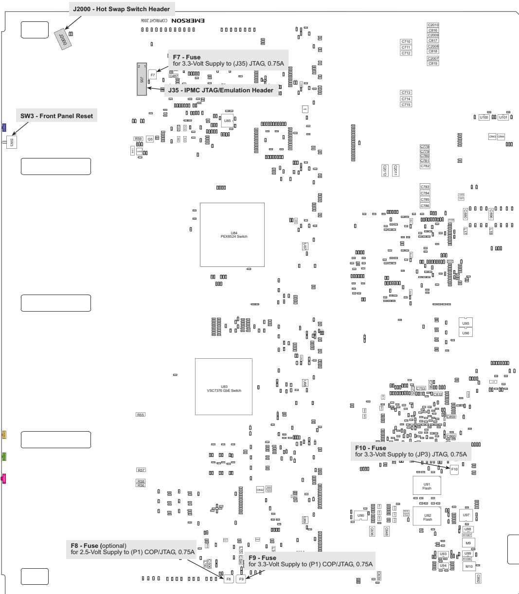
Figure 2-5: Jumper, Fuse and Switch Locations, Bottom
